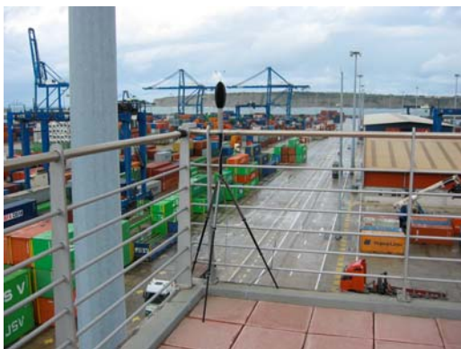
Figure #6: No screenings between the receivers and the noise source.
