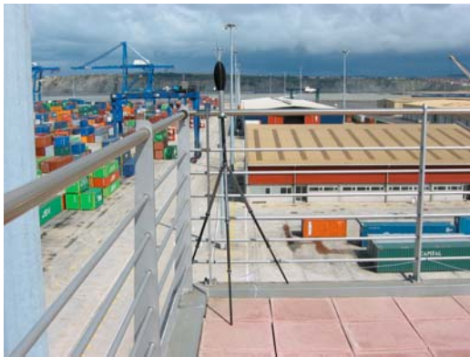
Figure #8: Receiving equipment with direct reflection effects.
