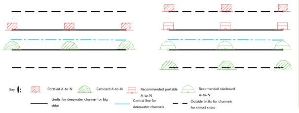
Figure 3: Two solutions to mark compound channels by visual AtoN
