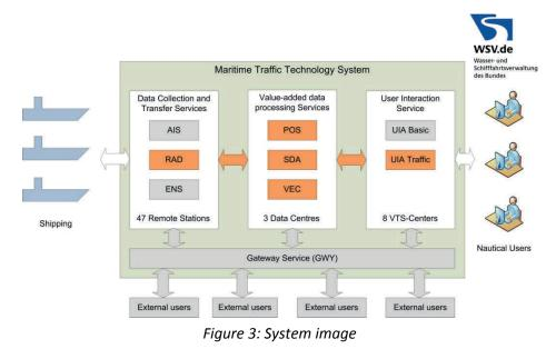
stations will be equipped with new sensors. The data of the stations are coastal wide merged in the data centres called "nodes" and are available for all users.
