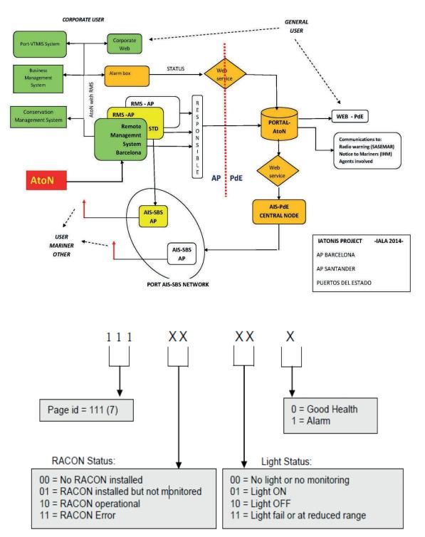
Figure 3 Recommended use of AtoN status bits
