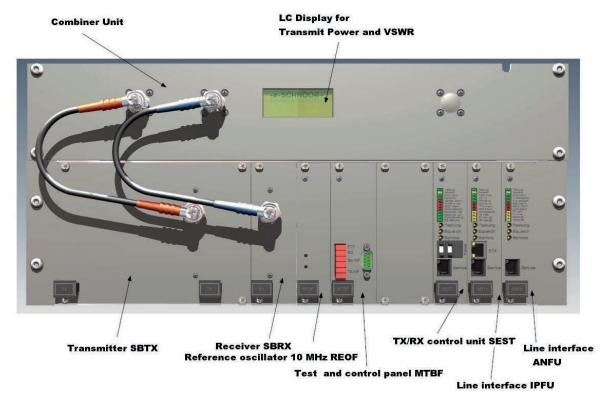
Figure 4: SEACOM radio with dual interfaces (bottom right of radio): IPFU to support IP connection and ANFU to support 4-wire analog connection
