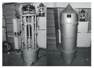
Figure 4: One colour, one position laser leading beacon : left – without mantle, - right – as an assembly
