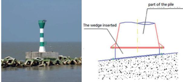
Figure 6: Solution for sedimentation of light beacon base along the guiding dikes
