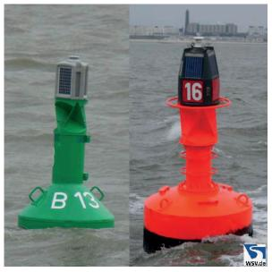
Figure 1: Buoys with IPSL and SKA
