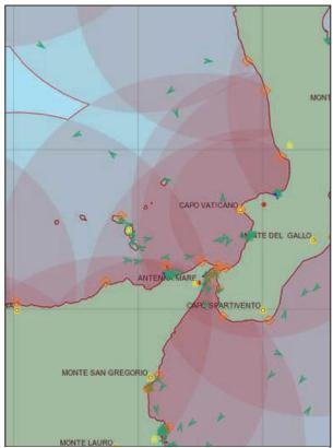
Figure 1 – AIS base stations coverage overlapping
