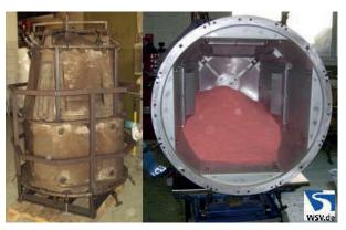
*Figure 6: Mould for upper housing*
