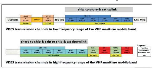
Figure 2: Example of channel designation for VDES in the VHF maritime mobile band
