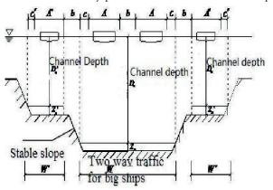
Figure 2: The cross section of compound navigation channels
