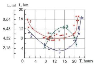
Figure 3: Results of comparison experimental detectable distances at marine observations (dots, circles and crosses) of the laser AtoNs (1), regular marine lights (2) and unlitmarks (3) as a day time function with MaexPro calculations (broken curves) at meteorological optical range equal 8 km.
