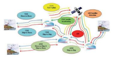
Figure 1: VDES functions for data exchange between ships, shore and satellite
