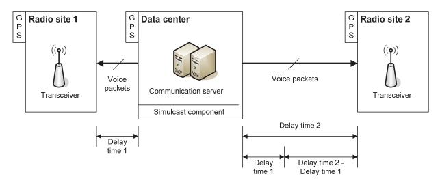
Figure 3: Principle of simulcast transmission
