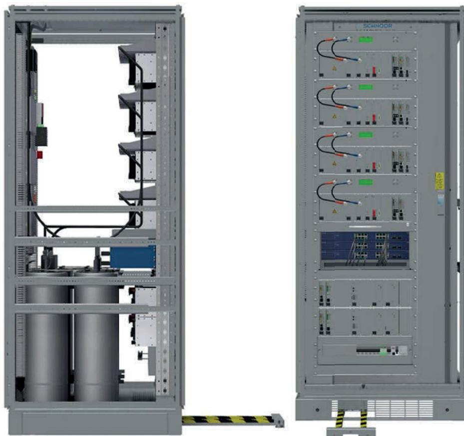
*Figure 3 : Radio base station rack with 4 transmitters/receivers, redundant power supplies and control Equipment. Antenna filter visible on side view (required if channel 16 and 70 are used with single antenna installation)*
