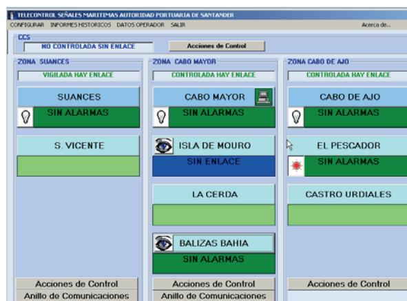
The installation of a remote monitoring system, which initially covered only eight lighthouses, began in the 1990's. This was an important step because it meant that not only were the lighthouses automated, but also that the AtoN Department of the Santander Port Authority had real-time information available on what was happening at each lighthouse.
