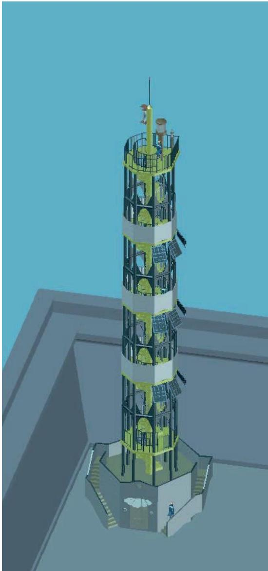
Reinforced concrete base-house, where the basic equipment for security, monitoring and supply, is been sheltered and protected.
