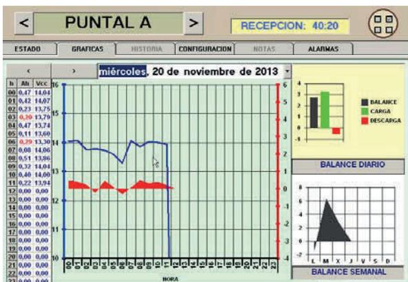
Due to the power constraints in these kinds of signals, a radio transmission system was carefully designed to take this aspect into account, so that it consumed as little power as possible. In this regard, the number of messages was limited to a maximum of four per hour, and one per hour was set by default. The capturing and transmission of analogue status signals was also implemented in
