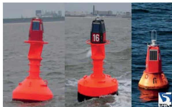
Figure 7: Comparison of LT81 with coloured and grey housing, FWT with coloured housing
