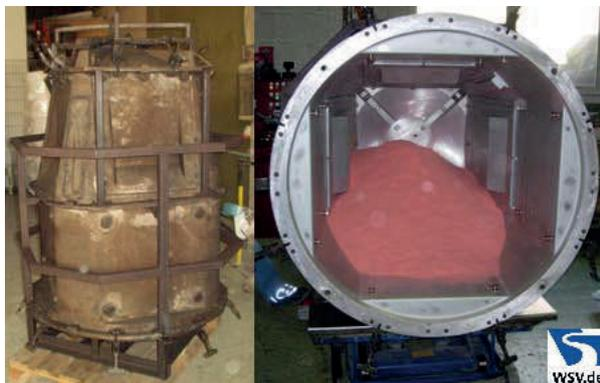
Figure 6: Mould for upper housing
