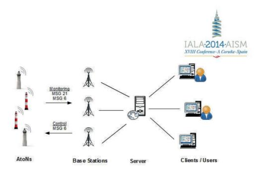
STAN program was carried out thanks a solution provided by McMurdo company. The hardware consists of KanAtoN3 and ComAtoN which are installed onboard the AtoN. The ComAtoN allows the acquisition and the processing of the status parameters and commands. The KanAtoN3 allows the transmission and the reception of the parameters on the VDL. VigieAtoN is the software which is a SCADA dedicated to the processing and to the analysis of messages 21, 6, 8 and 4.
