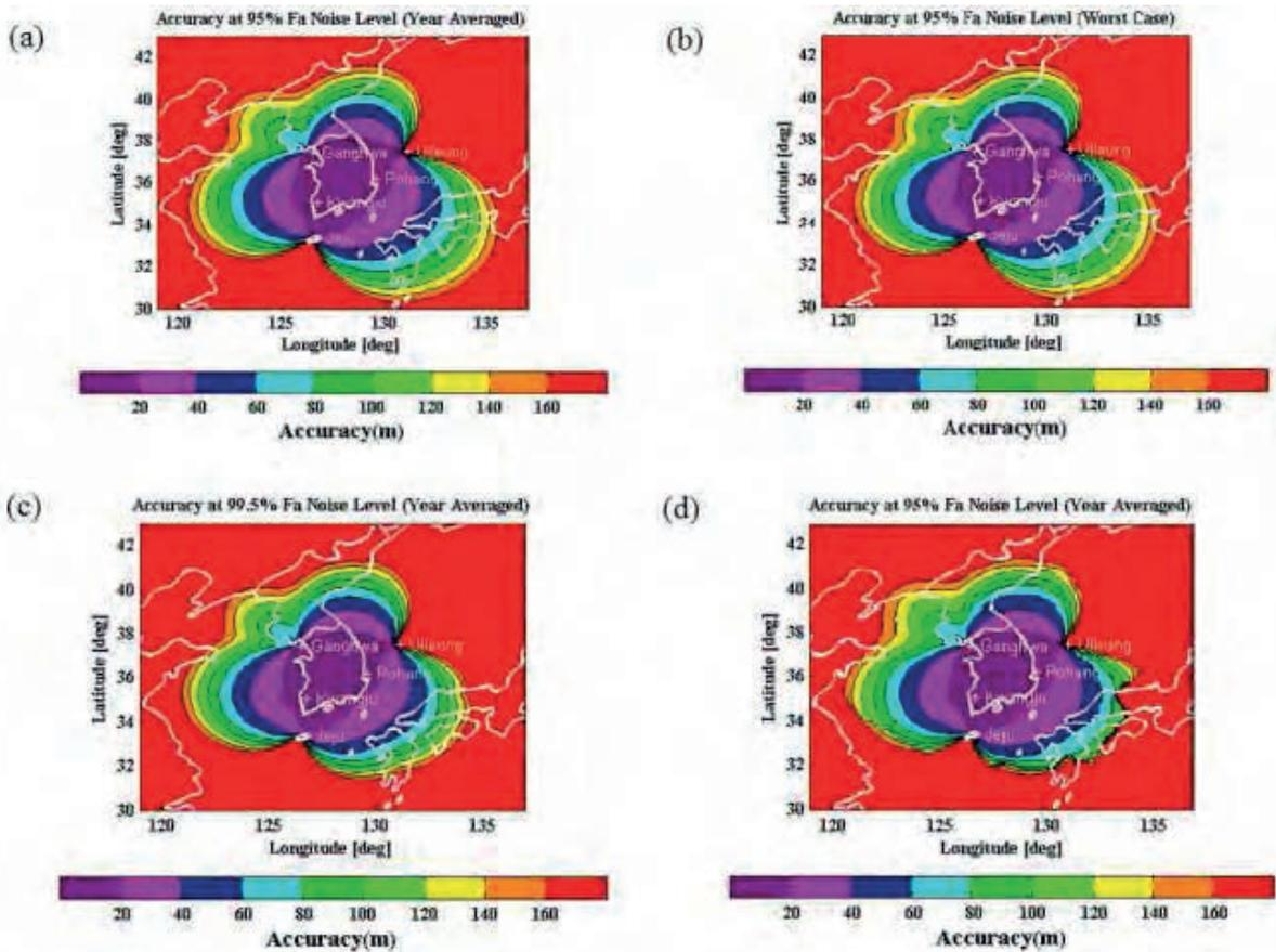
**FIGURE 5:** Example accuracy simulation results for various conditions (a) Repeatable accuracy plot for 95% noise level, year averaged, -15dB of SNR threshold (b) Repeatable accuracy plot for 95% noise level, worst case of a year, -15dB of SNR threshold (c) Repeatable accuracy plot for 99.5% noise level, year averaged, -15dB of SNR threshold (d) Repeatable accuracy plot for 95% noise level, year averaged, -12dB of SNR threshold
