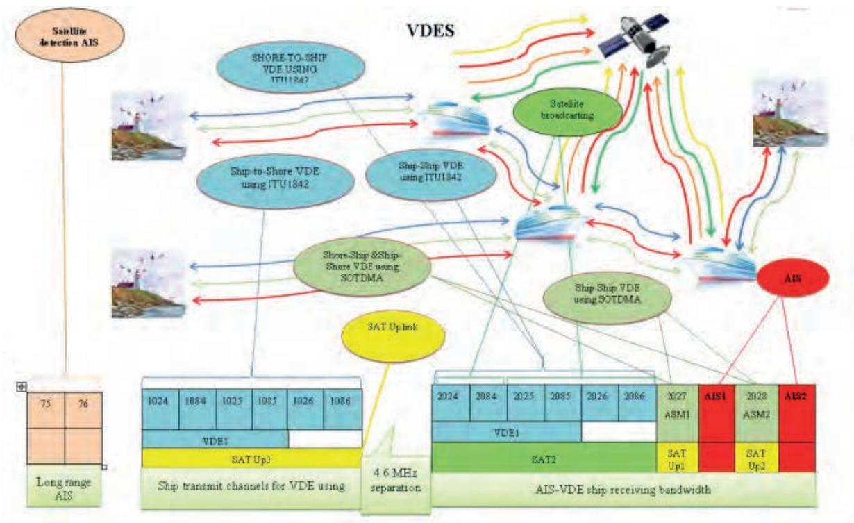
FIGURE 1: VDES Functions and Frequency Usage
