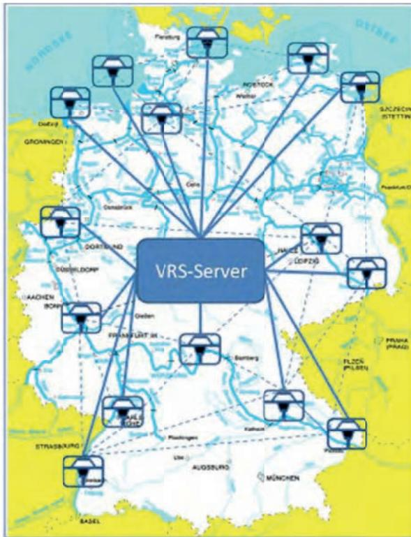
Figure 1: Example of a VRS-network in Germany
