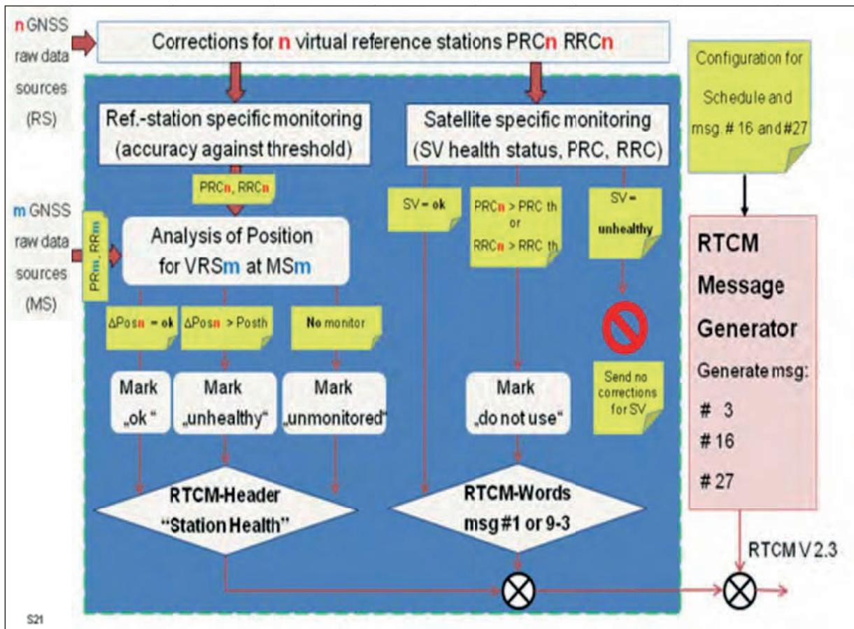
Figure 2: Pre Broadcast Monitoring (PBM) as part of the VRS-Server
