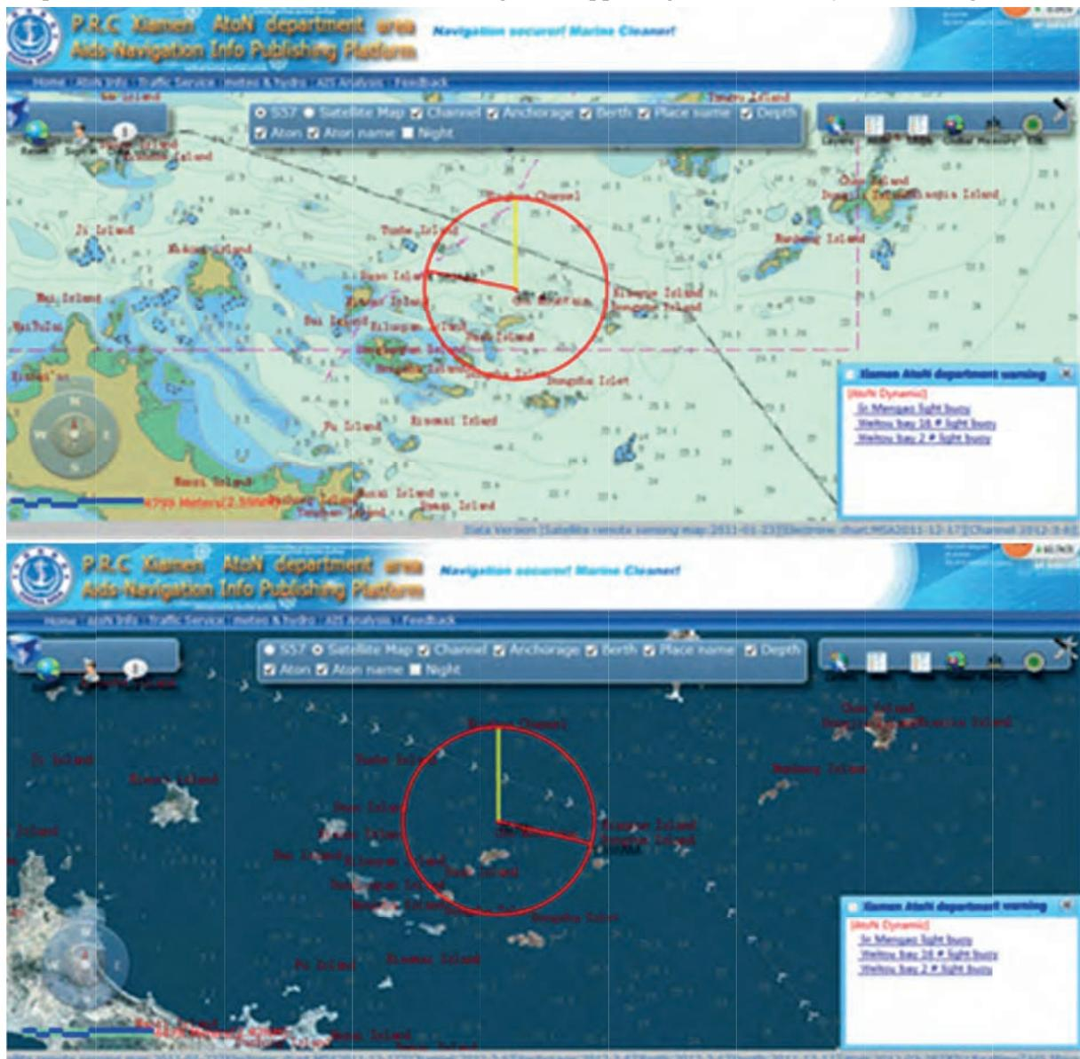
Figure 6: Systems interface based on S-57 ECDIS and Satellite remote sensing
