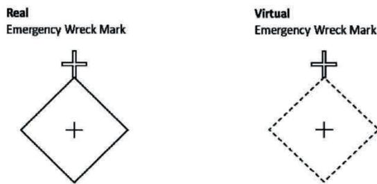
Figure 4: Draft new symbols for AIS AtoN of Emergency Wreck Mark
