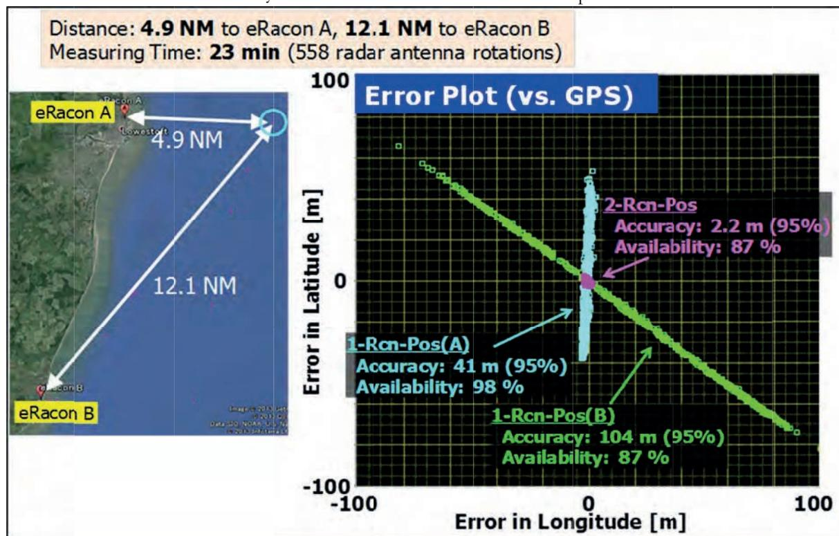
Figure 7: Results of the Absolute Radar Positioning trials in the UK.
