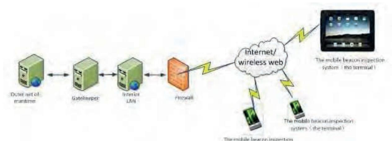
Figure 7 : Network architecture of mobile Beacon inspection technology
