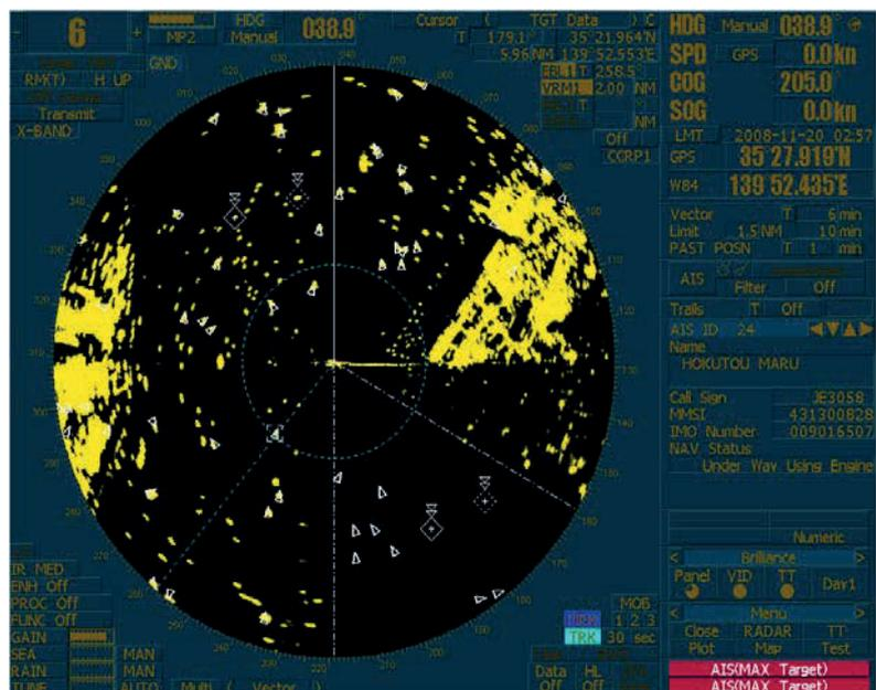
Figure 3: Radar simulator display (XGA)
