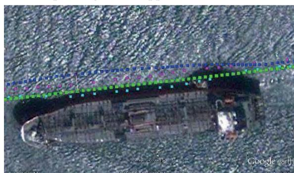
Figure 3: Google Earth plot with the position updates from each of the devices and the PosMV truth position; Samsung (dark blue), iPhone (magenta), iPad (cyan) and Pos MV truth (green)
