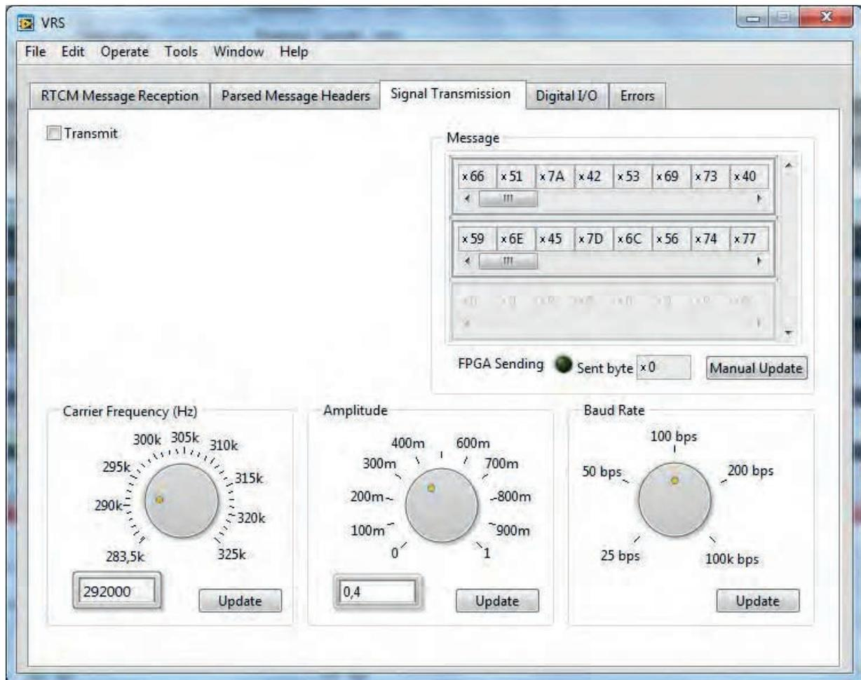
Figure 8: GUI for the MSK modulator
