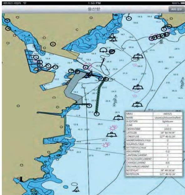
Figure 4 Snapshot of AtoN data overlaid onto ENC
