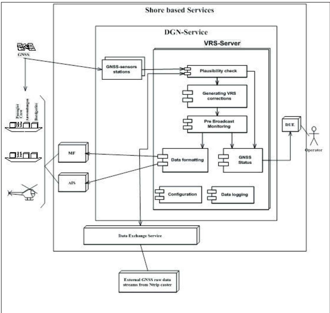
Figure 5: VRS concept based on new shore based services (DGN, MW and AIS)
