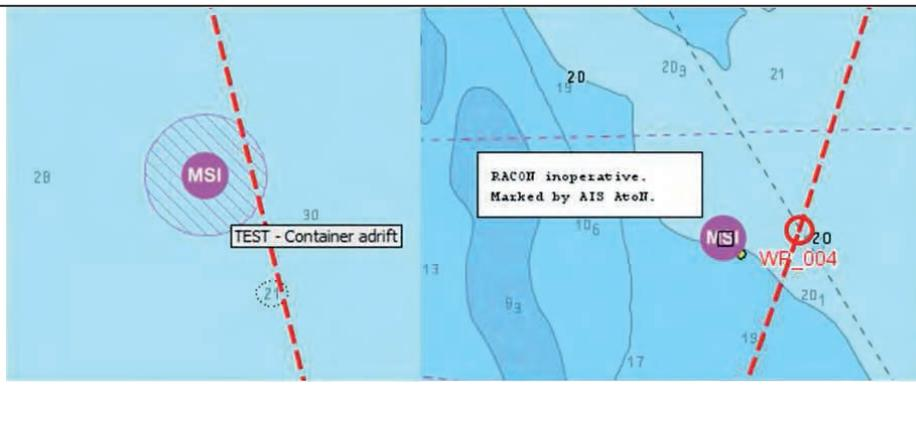
Figure 6: Example of the MSI/NM service on the electronic chart system
