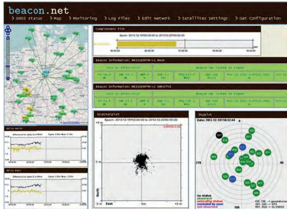
Figure 4: graphical user interface of the VRS software which runs at the VRS test pilot
