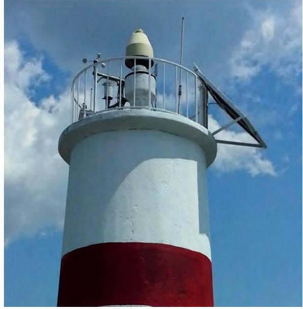
Picture 5: SOTAS with automatic meteorological D-OMGI
