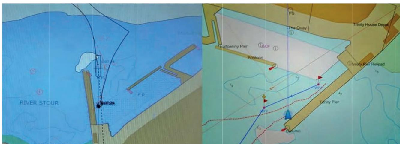
Figure 2: Comparison of the vessel's ECDIS display (left) compared to the iPad display (right) as the vessel approached the quay. The iPad display shows an incorrect vessel heading
