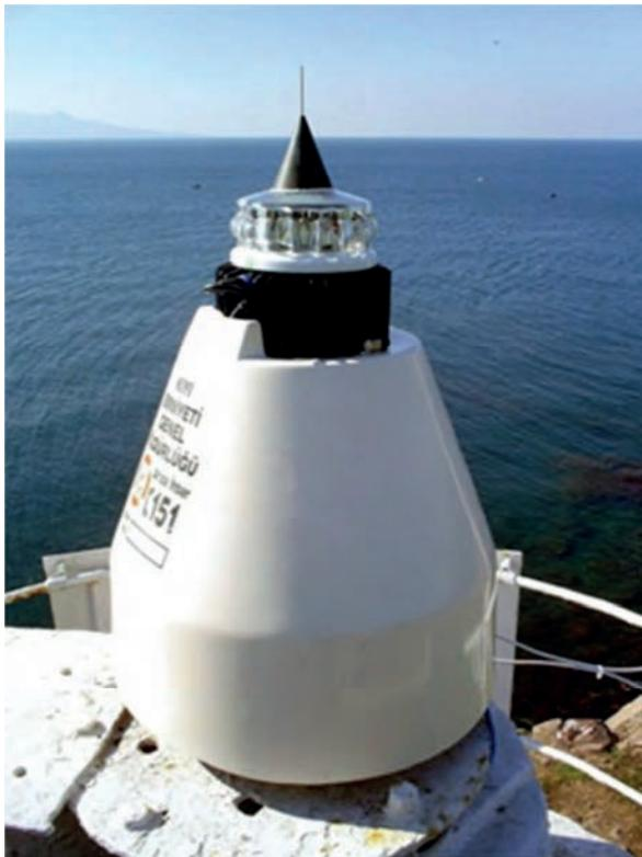
Picture 9: SOTAS station with 10 nm LED lantern
