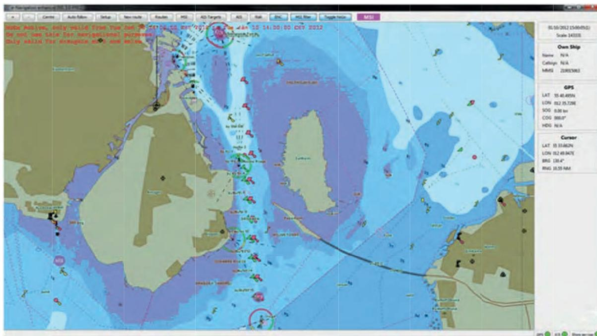
Figure 5: Example of the no-go area e-Navigation service. The purple shading shows the area that the vessel should not enter due to insufficient under-keel clearance
