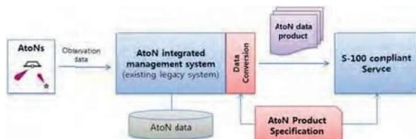
Figure 7 Diagram of AtoN data conversion process
