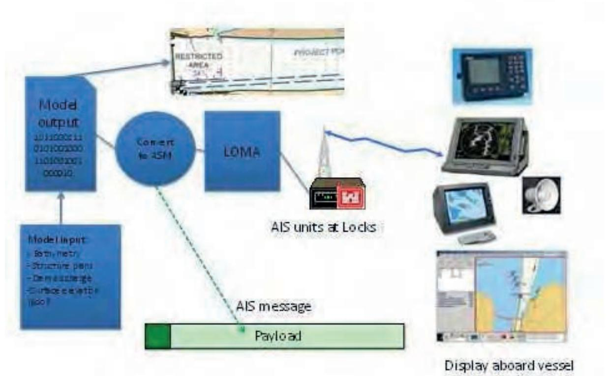
Figure 1. Lock approach current model information via AIS
