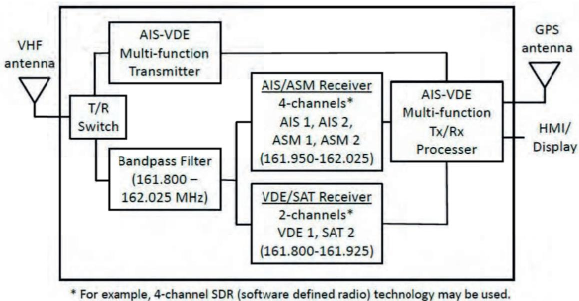
FIGURE 2: Example VDES Functional Diagram
