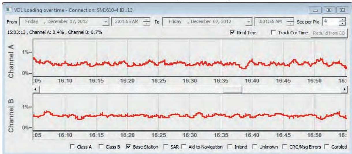
Figure 2: VDL loading for base stations only
