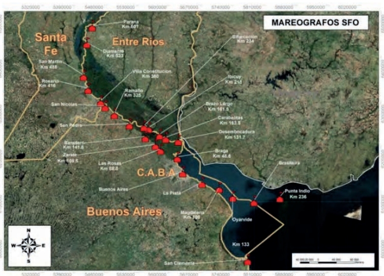
Figure 3: Water level/meteorological measuring stations – 24 stations from Santa Fe to the Ocean
