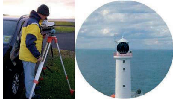
Figure 13: Left: Setting up the photometer; Right: A typical view through the eyepiece of the Hagner S4, the dark centre is the measurement field
