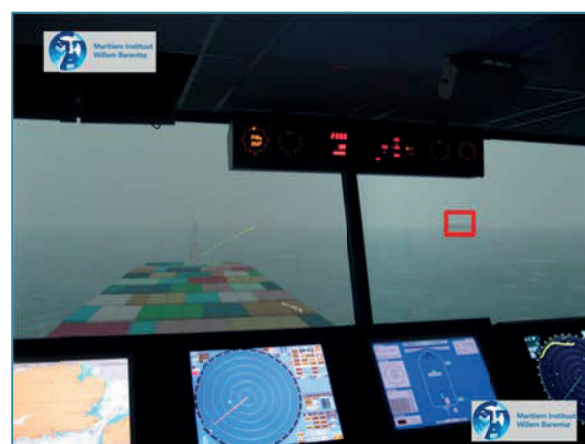
Figure 7: Conceptual Study for Portrayal of a vessel’s route based on the RTM data to the bridge team using Head-Up-Display portrayal mode (dotted line) [Ongoing work within the ACCSEAS WP4 MSP-Stream; courtesy Maritiem Instituut Willem Barentsz, Mr. Stephan Procee]
