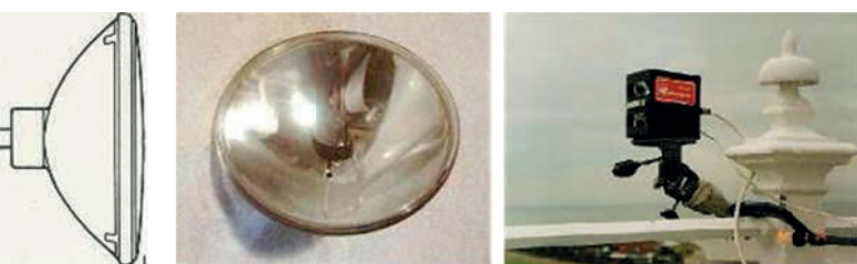
Figure 5: Left: Outline drawing of a typical sealed beam lamp; Centre GE Q4559X; Right: 'Red' reference light mounted on gallery
