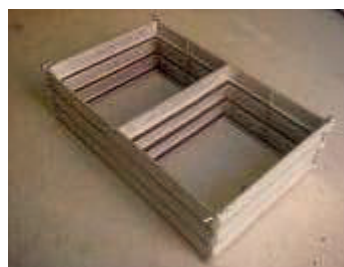
Figure 6: Three part prism frame collapsed for transportation
