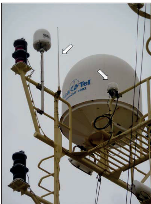
Figure 4: Close-up of the AIS AtoN installation on THV Alert.
