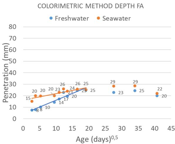
Figure 8. Chloride depth. Fly ash cement (CEM II), 2023. Square root of time
