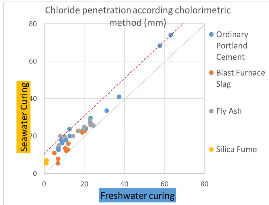
Figure 10. Chloride penetration according to colorimetric method in freshwater and seawater-cured concrete (2022 and 2009)
