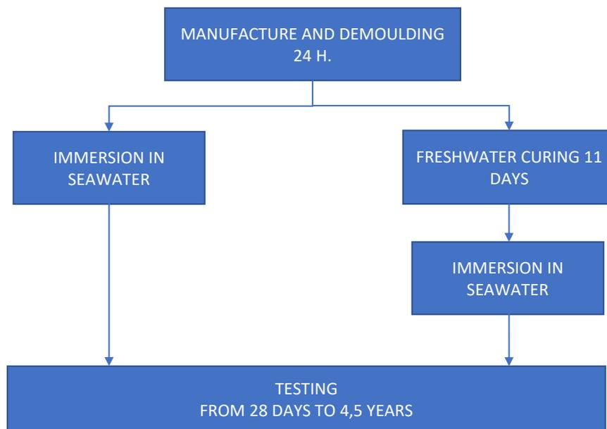
Figure 1. Different curing methods implemented in laboratory study
