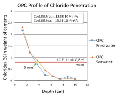
Figure 11. Profile of chloride concentration in OPC (1 year). 2022
