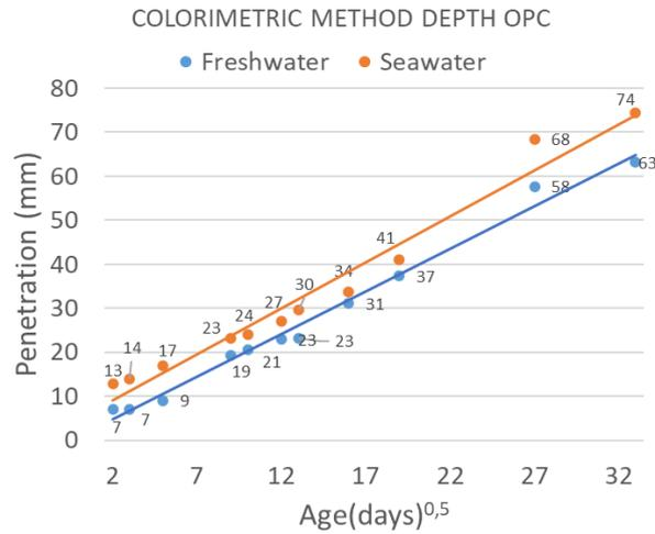
Figure 7. Chloride depth. Ordinary Portland cement (CEM I), 2023. Square root of time
