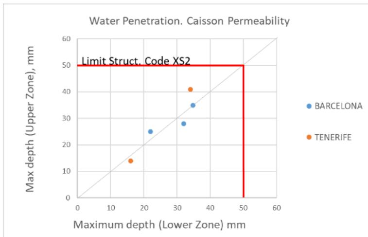
Figure 21. Permeability of concrete. Comparison of UPPER and LOWER concrete
