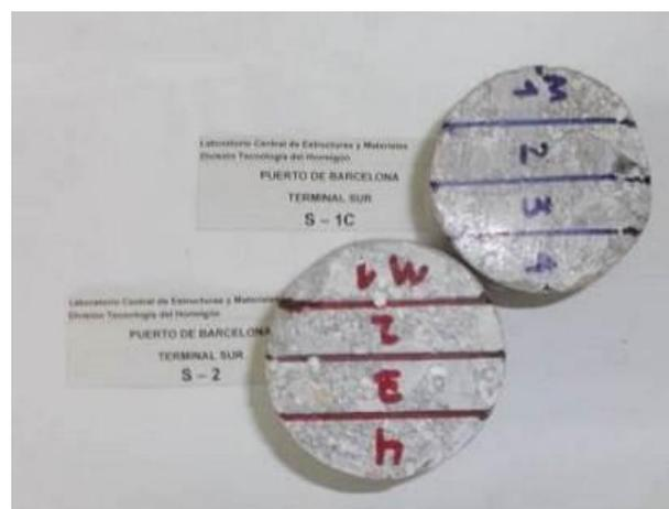
Photograph 11. Preparation of samples for the chloride profile
