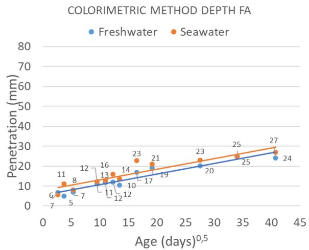
Figure 9. Chloride depth. Blast-furnace slag cement (CEM III), 2023. Square root of time
