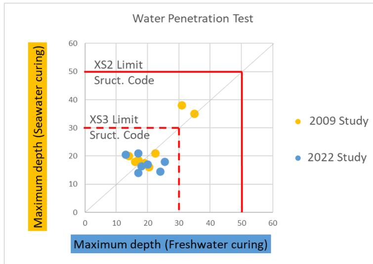
Figure 3. Maximum water penetration depth. Seawater and freshwater curing. 2009 and 2022 research
