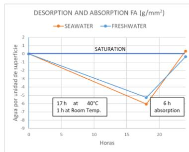
Figure 16. Capillary absorption to saturation, desorption 17h at 40°C and 6 hours absorption for FA
