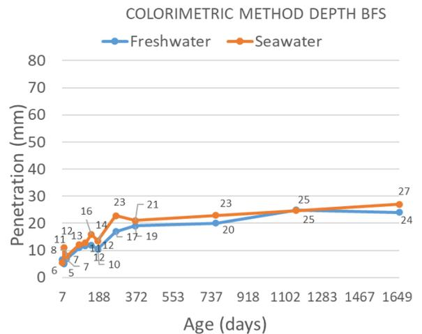
Figure 6. Chloride depth. Blast-furnace slag cement (CEM III). 2023
