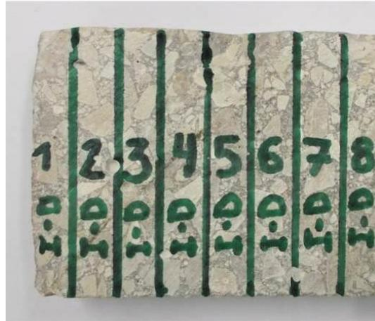
Photograph 5. Sample for chloride profile testing. Each band is cut and analysed to determine the chloride content
