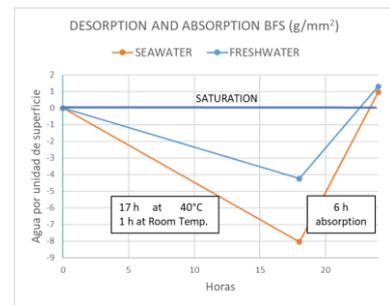
Figure 17. Capillary absorption to saturation, desorption 17h at 40°C and 6 hours absorption for BFS
