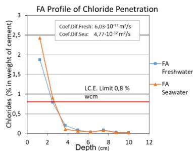
Figure 12. Profile of chloride concentration in FA (1 year). 2022
