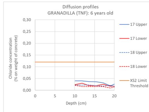
Figure 23. Chloride diffusion profiles. Caissons from Tenerife Harbour. Comparison of UPPER and LOWER concrete
