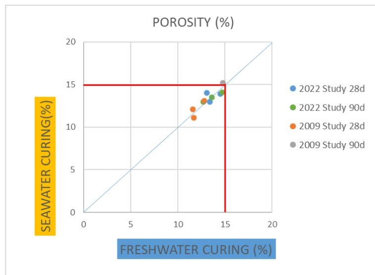
Figure 14. Results of porosity in XY graph for the different types of curing and age of the samples
