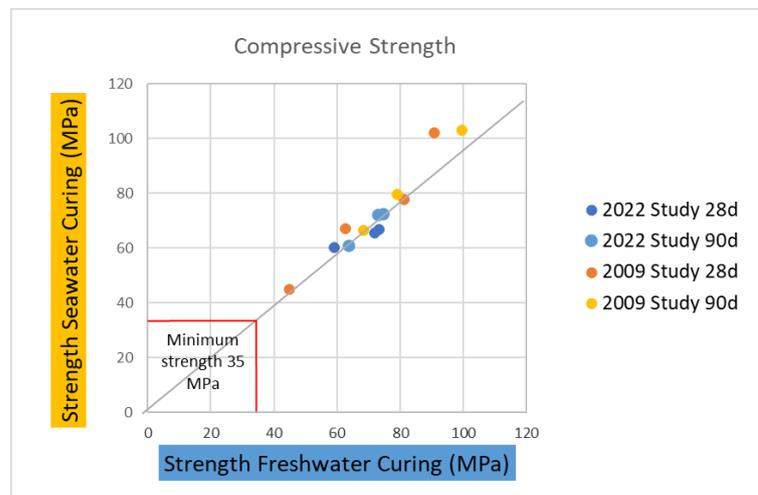
Figure 2. Compressive strength, comparing seawater and freshwater curing methods. 2009 and 2022 research
