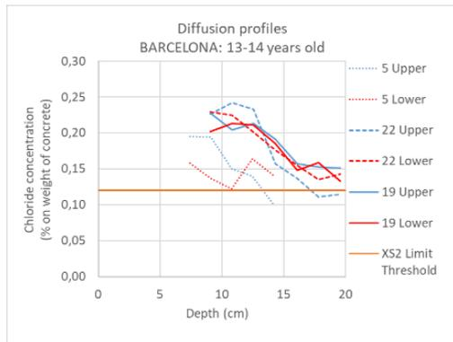
Figure 22. Chloride diffusion profiles. Caissons from Barcelona Harbour. Comparison of UPPER and LOWER concrete
