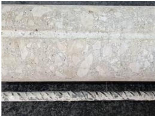
Photograph 12. Vertical reinforcement without corrosion. Caisson D. Barcelona Port
