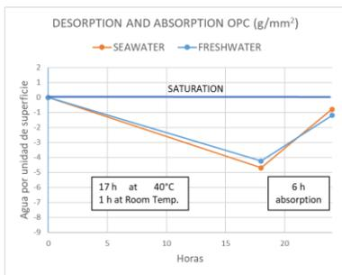
Figure 15. Capillary absorption to saturation, desorption 17h at 40°C and 6 hours absorption for OPC
