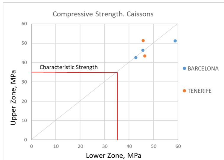
Figure 20. Compressive Strength. Comparison of UPPER and LOWER concrete
