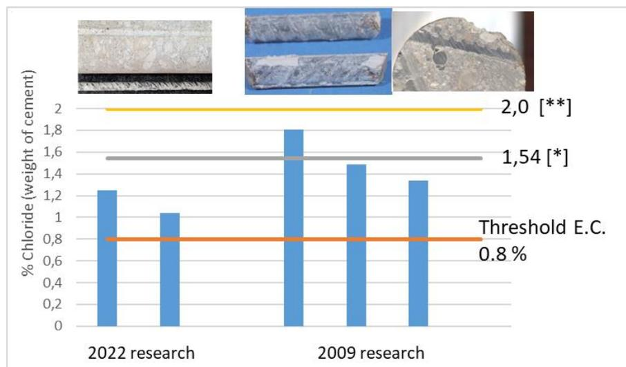
[\*] Threshold for concrete in an XS2 environment. [20]
