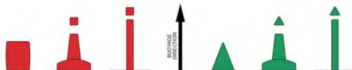
Figure 1 Lateral marks used in Region A
