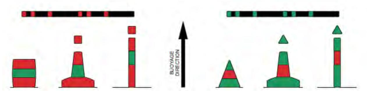
Figure 3 Preferred Channel marks used in Region A
