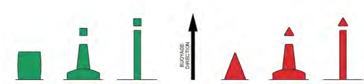
Figure 2 Lateral marks used in Region B
